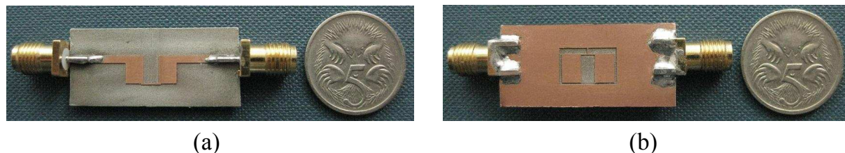
Figure 3.15. The fabricated dual-mode bandstop filter. The fabricated filter prototype. (a) Top view. (b) Bottom view.
