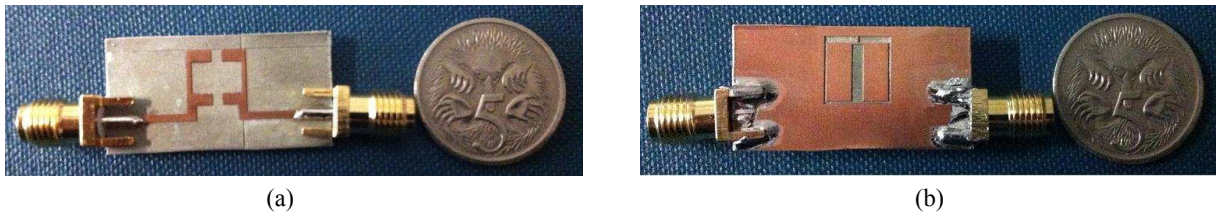
Figure 3.8. Fabricated prototype of the dual-mode filter. Top view (a) and bottom view (b) of the fabricated filter prototype.
