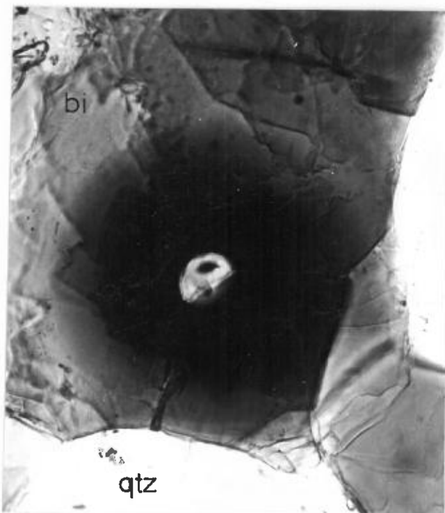
Fig. 8. Pleochroic halo around minute zircon in biotite grain. Spec. C1. Transmitted light. x450.
