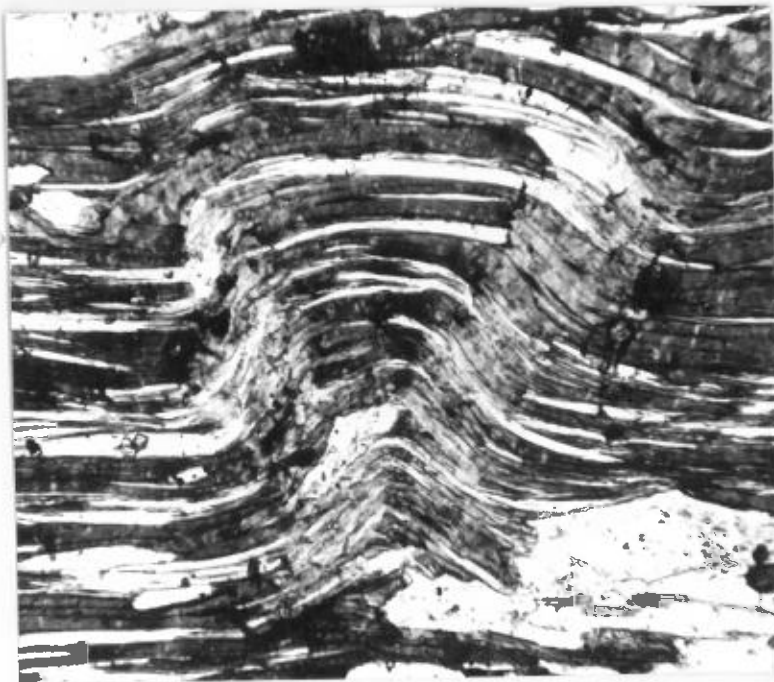
Fig. 28(b). Conjugate set of fine kinks. Spec. C8. Transmitted light. x75.
