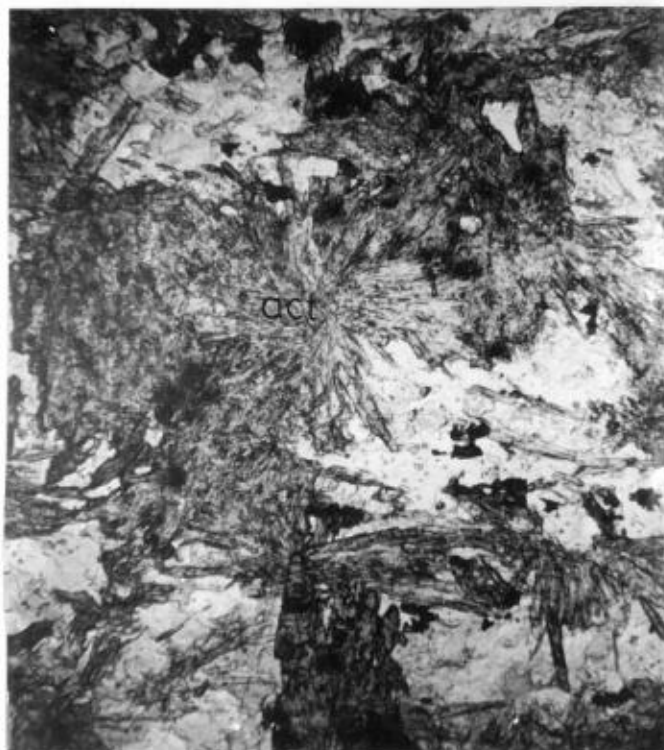
Fig. 17. Amphibolite showing radiating actinolite in feldspar-quartz matrix. Spec. B33. Transmitted light. x75.
