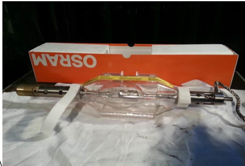
Figure 4.10 Photograph of the HLR Osram 5kW Xenon short-arc lamp used in the experiment.
